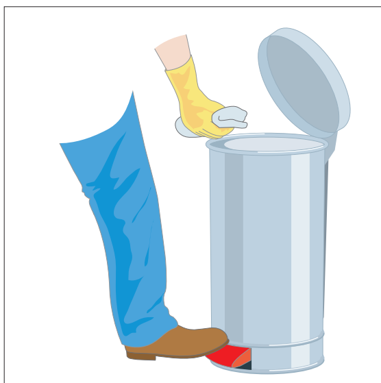
Figure 23: A fire-resisting pedal bin for rags
